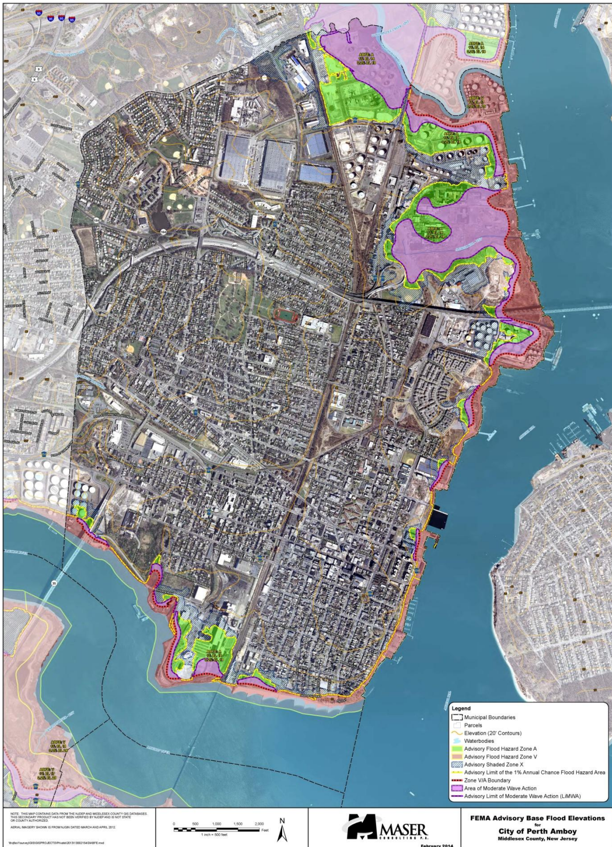
Figure 14: Advisory Base Flood Elevation Map (2013) of Perth Amboy showing large areas of "moderate wave action".
